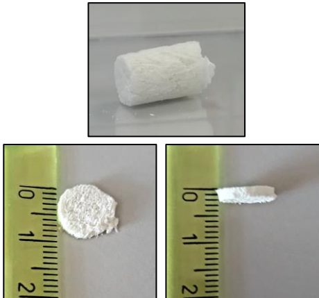
3D Scaffold Collagen I - Hydroxyapatite (30:70 ratio)
